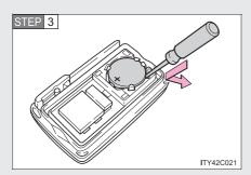
Remove the depleted battery.
