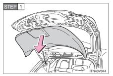
Open the back door and remove the trim board.
