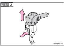
Unplug the connector while pushing the lock release.
