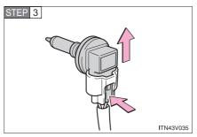
Unplug the connector while pushing the lock release.
