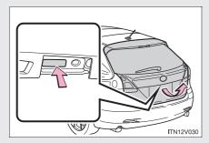
Raise the back door while pushing up the back door opener switch.
