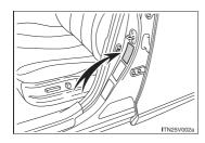
For the GAWR, see the Certification Label. For the maximum load of the tire, see the load limit at maximum cold tire inflation pressure mentioned on the sidewall of the tire.  $(\rightarrow P. 498)$
