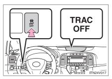
To turn the TRAC system off, quickly press and release
