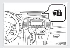
Close the doors and hood, and lock all doors using the entry function (vehicles with smart key system) or the wireless remote control. The system will be set automatically after 30 seconds.
