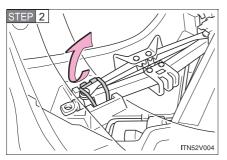
Unlock the tightening strap.
