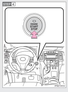
Press the "ENGINE START STOP" switch.
