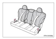
Fold down the seatback while pulling the seatback angle adjustment lever.
