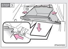
Push each side of the glove box to release the pins. Then disconnect the claws at the bottom and remove the glove box.
