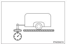
The load placed on the trailer hitch ball. ( $\rightarrow$ P. 264)
