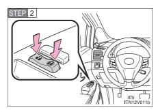
Shift the shift lever to "P" or "N", press and hold the driver's door lock switch ( or ) for about 5 seconds then release.
