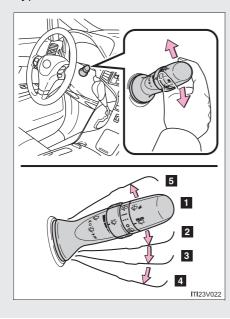
Off 1 Intermittent wiper 2 💭 operation Low speed wiper 3 operation High speed wiper operation Temporary operation 5
