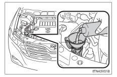
If any washer does not work or the low windshield washer fluid level warning light comes on, the washer tank may be empty. Add washer fluid.
