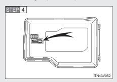
Remove the fuse with the pullout tool.
