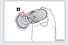
Wash/wipe operationWipers operate automatically.
