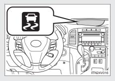
To engage hill-start assist control, further depress the brake pedal when the vehicle is stopped completely.
