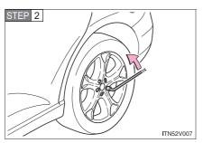
Slightly loosen the wheel nuts (one turn).
