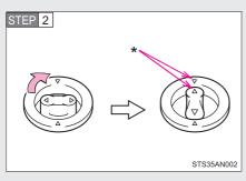
Turn the upper knob of each retaining hook (clip) to secure the floor mats in place.
